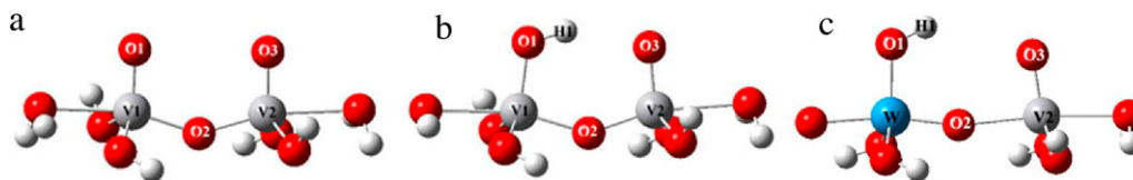
Fig. 1. The optimized structure of the cluster (a) V_2O_9H_8 ; the structure of the optimized Brønsted acidic (b) V_2O_9H_8 cluster and (c) VWO_9H_7 cluster.
